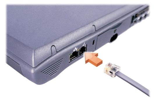
If your computer has an internal modem, connect the telephone cable to the internal modem connector. If the connector has a plastic cover, your computer does not have an internal modem; check for a PC Card modem.
