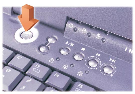
Press the power button to turn on the computer. **HINT:** The touch pad does not work when you first start the computer. Press a key when
